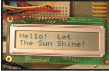
Photo 4—The data logger greets users before leading them through the system setup.
