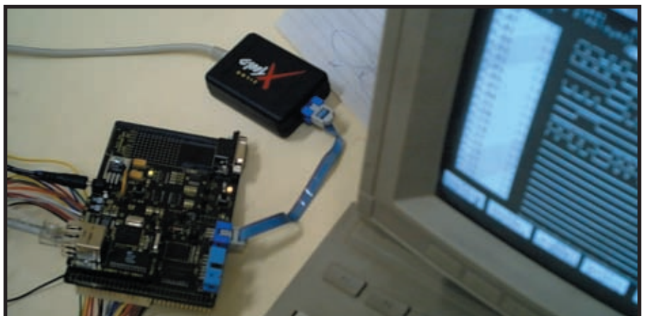
Photo 1 —Take a look at the Arby with the programming interface used during the project development stages. The system generated the waveforms on the logic analyzer.
