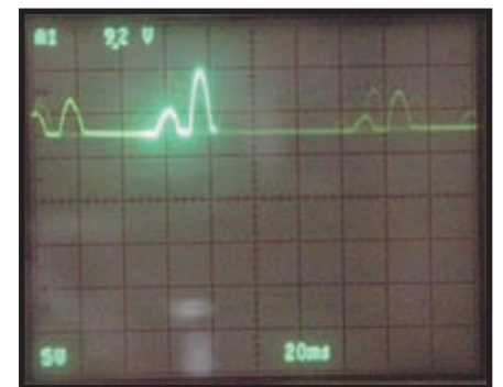
Photo 3 —When shaken, an internal magnet slides back and forth through the coil. The coil produces voltage pulses as the magnetic field cuts through the coil's winding. This voltage pumps up a supercapacitor, which is the power source for a single LED.
