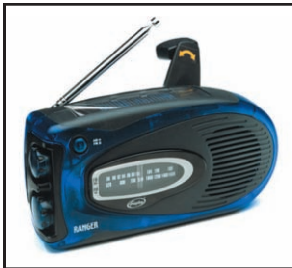
Photo 1 —Freeplay’s Ranger radio has multiple charging sources. Its AAA NiMH batteries can be charged from the AC adapter, the internal alternator’s cranking handle, or an internal solar cell. The operating time is about 5 to 50 times the cranking time (depending on crank RPM and playback volume).
